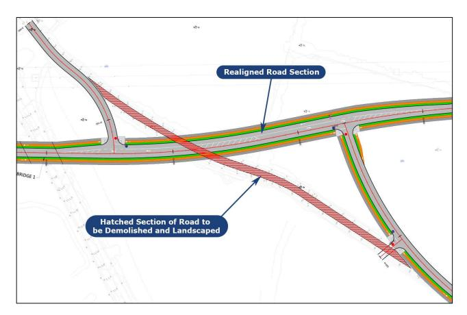
Figure 7: Road Section to be Realigned
