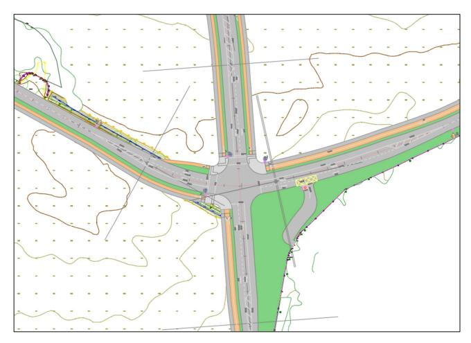
Figure 9: Realigned Signalised Junction on Eastern
